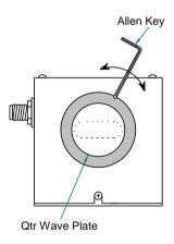
NOTE. For the **LS110 XY**, the waveplates are secured with locking screws. Remove cover to gain access.
